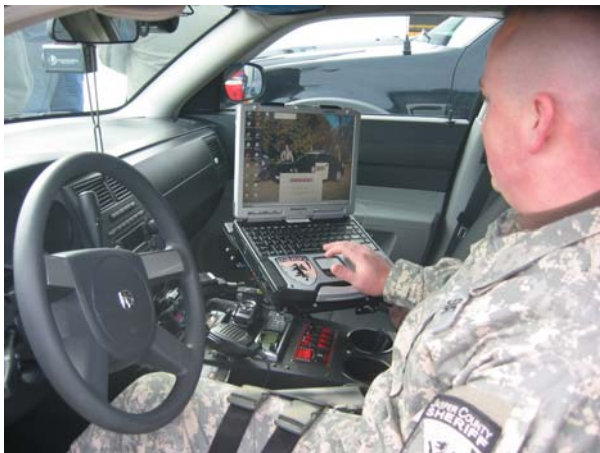
Mobile data terminals, like this one in the Jasper County Sheriff’s Department, lets officers receive and send data.
